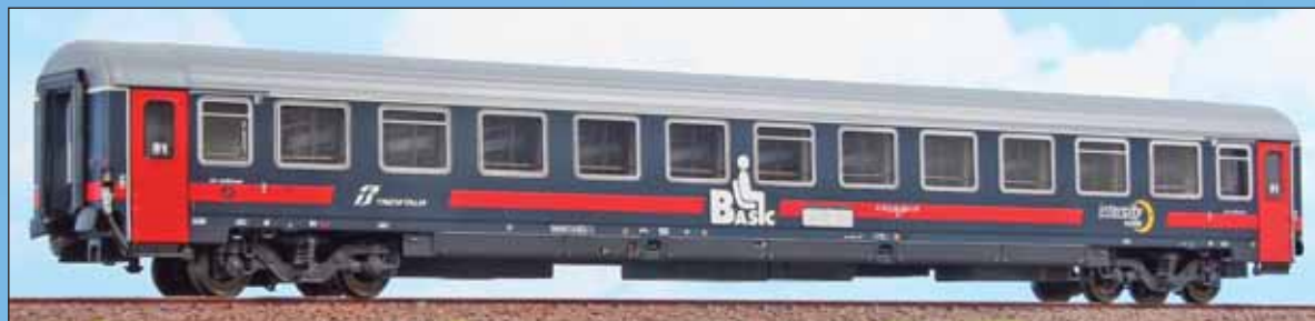
Carrozza UIC-Z "Basic" con posti a sedere, in livrea "Intercity Notte" attuale di Trenitalia. Type UIC-Z "Basic" car in actual Trenitalia "Intercity Notte" livery. Typ UIC-Z "Basic" wagen in aktueller "Intercity Notte"-Lackierung.
